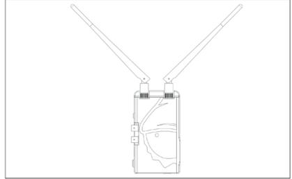
Position the antennas on transmitter as shown in the illustration. This ensures the best possible RF performance.
